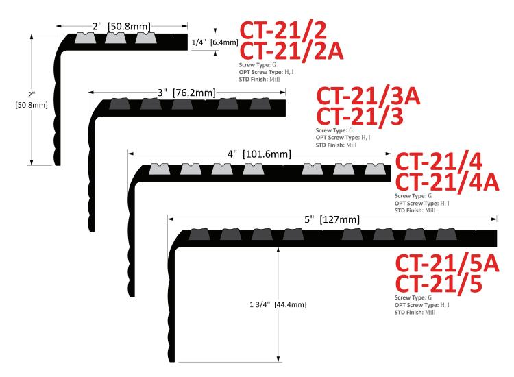
AVAILABLE WITH LANEL P.V.C. INSERT OR ALUMINUM OXIDE GRIT IN EPOXY BASE ABRASIVE (A). STAIR NOSINGS ARE SUPPLIED WITH COUNTERSUNK HOLES AND TAPCON SCREWS.
